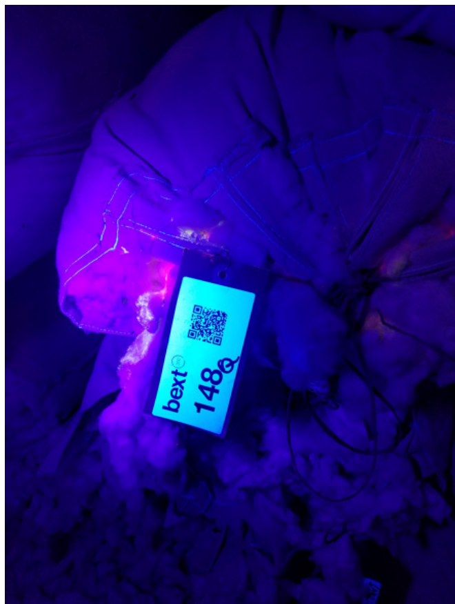
Figure 5: The IN-Code fluorescent marker identified using a UV flashlight.
